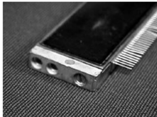
Figure 7 Microwave package close-up of drilled and tapped gas purge port (R). The left two ports are co-axial feedthrus.
