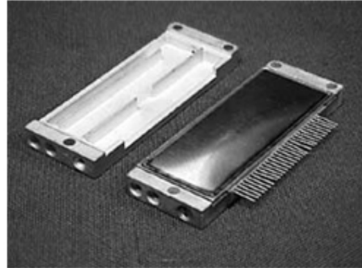
Figure 6 Ni-Au Plated AlSiC microwave package (L), and integrated, assembled, and sealed package (R).
