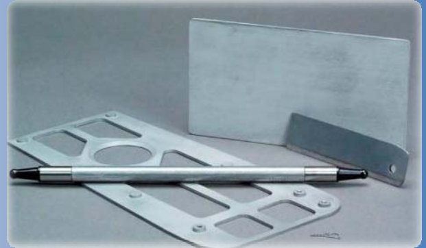
MMC composites are ideal for components that require stiffness, strength and light weight
